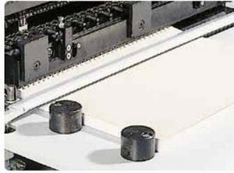
Automatic binding table clamps the media and holds the blocks in place during binding.
